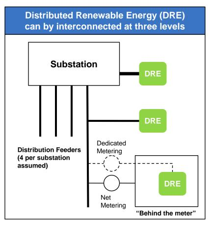
**Substation interconnection** means that the DRE is physically located close to the substation, and a dedicated electrical connection to the low side bus would be made.
