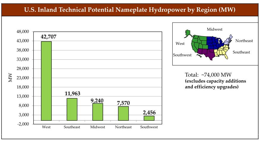
Source: INL Feasibility Assessment of the Water Energy Resources of the US for New Low Power and Small Hydro Classes of Hydroelectric Plants 2006 and Estimation of Economic Parameters of U.S. Hydropower Resources 2003: Excludes Capacity Additions and Efficiency Upgrades
