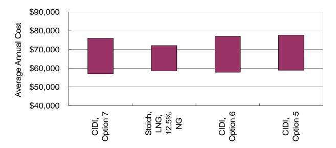
NOTE: In the figure above, "Option #" refers to aftertreatment combinations used in the ACC model. Option #5 consists of a regenerative PM trap, urea–SCR, and oxidation catalyst; Option #6 consists of a regenerative PM trap, sulfur trap, NO<sub>x</sub> trap, and oxidation catalyst; and Option #7 consists of a 4-way catalyst (see Table 3-1)
