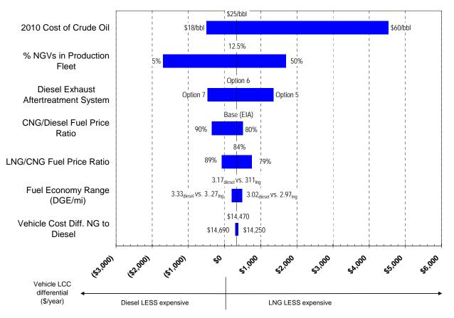
Figure 4-1. Refuse Hauler Application: LNG Compared to CIDI
