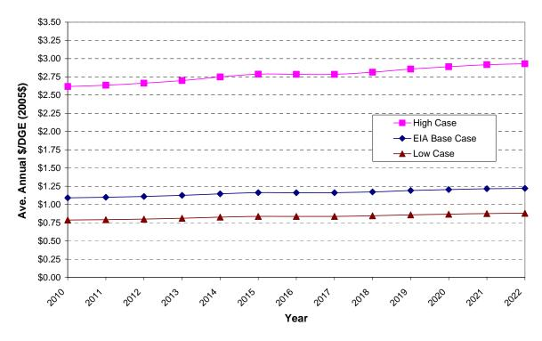
Figure 2-2. CNG Price Range used in the Analysis
