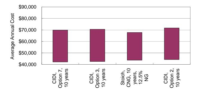
In the figure above, "Option #" refers to aftertreatment combinations used in the ACC model. Option #2 consists of catalyzed PM trap, SCR-urea, and oxidation catalyst; Option #3 consists of catalyzed PM trap, sulfur trap, NO<sub>x</sub> trap, and oxidation catalyst; and Option #7 consists of a 4-way catalyst (see Table 3-3)
