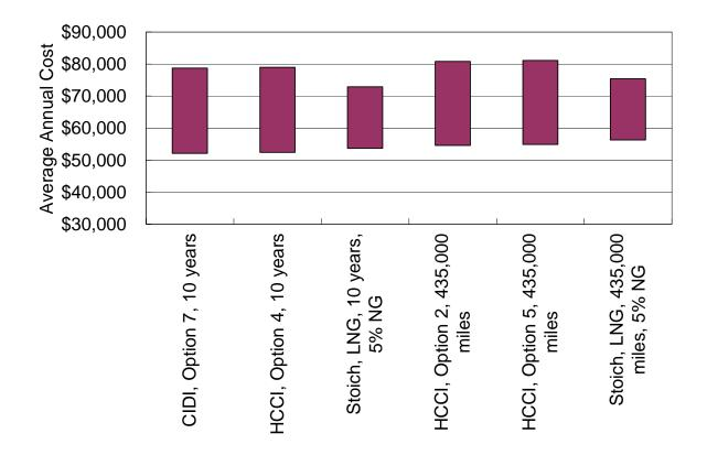
NOTE: In the figure above, "Option #" refers to aftertreatment combinations used in the ACC model. Option #2 consists of catalyzed PM trap, SCR-urea, and oxidation catalyst; Option #4 consists of regenerative PM trap, SCR-HC, and oxidation catalyst, Option #5 consists of regenerative PM trap, SCR-urea, and oxidation catalyst; and Option #7 consists of a 4-way catalyst (see Table 3-2).
