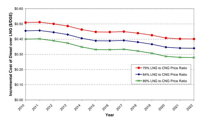
Figure 2-7. LNG Fuel Price Differential for Sensitivity Analysis
