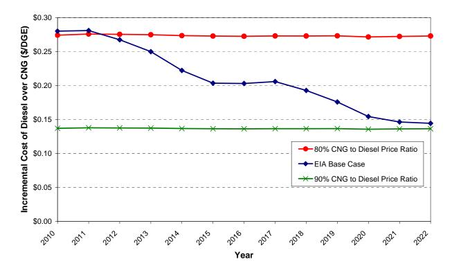
Figure 2-6. CNG Fuel Price Differential for Sensitivity Analysis
