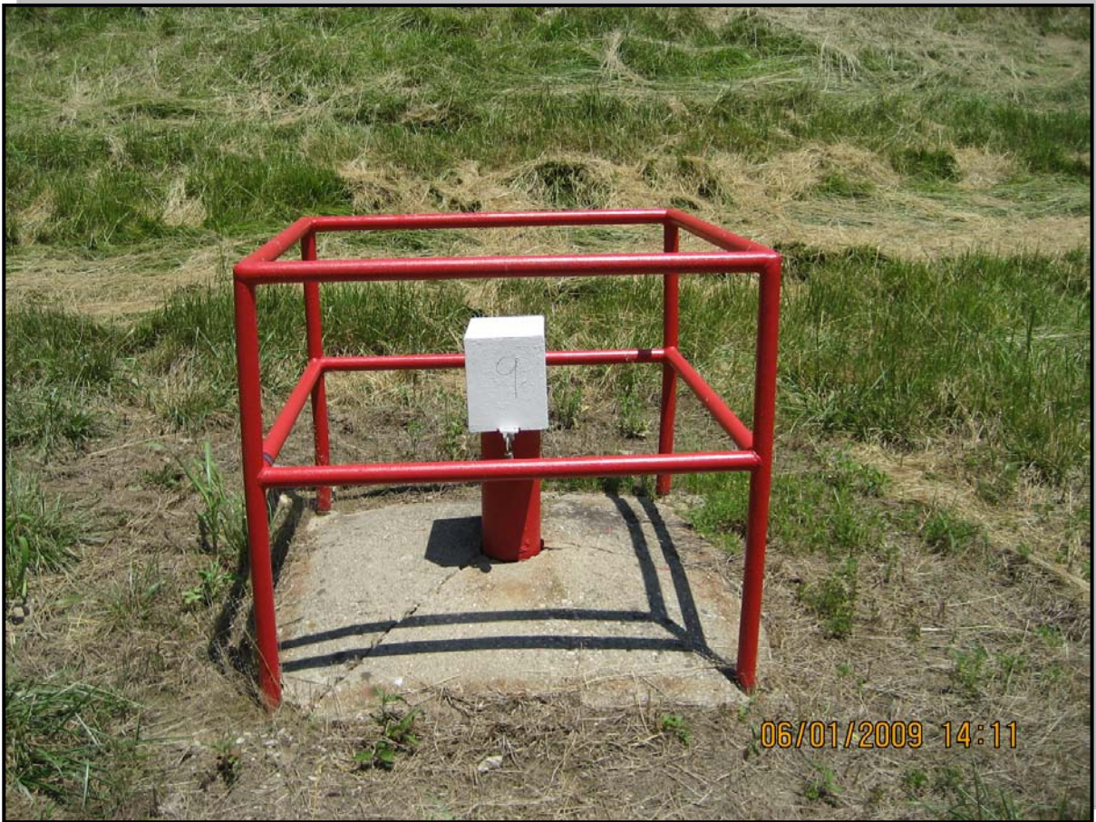
Photo 7 – Typical view of groundwater monitoring well (Not used for seepage or pore pressure monitoring)
