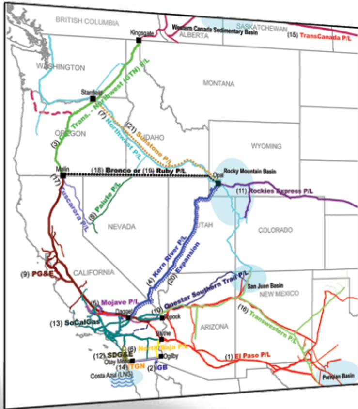
FIGURE 15: NATURAL GAS RESOURCE AREAS AND PIPELINES
