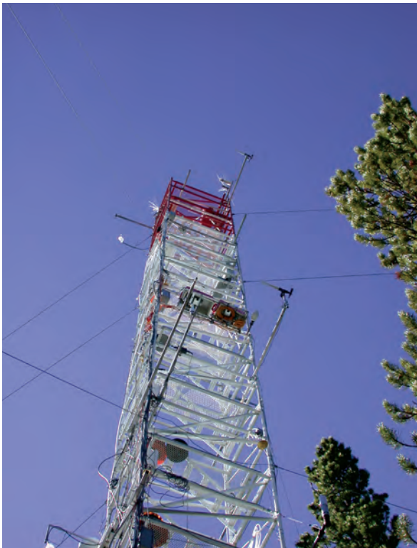
Figure 23. Instruments for measuring exchange of carbon dioxide and water between a forest and the atmosphere at the Niwot Ridge Long Term Ecological Research Site. (Image courtesy Michael G. Ryan.)
