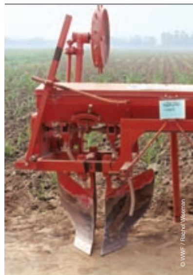
Ox drawn furrow ridger. The tube allows efficient application of fertiliser reducing cost and nutrient run-off.
