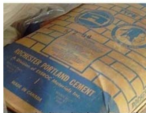
A sack of Portland cement will yield about 1.18 cu. ft. of cement
