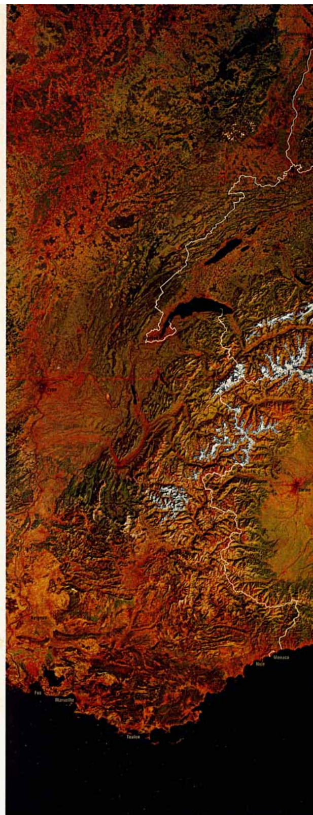
Figure 7. —Landsat image mosaic of the Alps at 1:3,300,000 scale. The mosaic was produced by the Georg Westermann Company, Braunschweig, Germany. Parts of 50 Landsat images were used.
