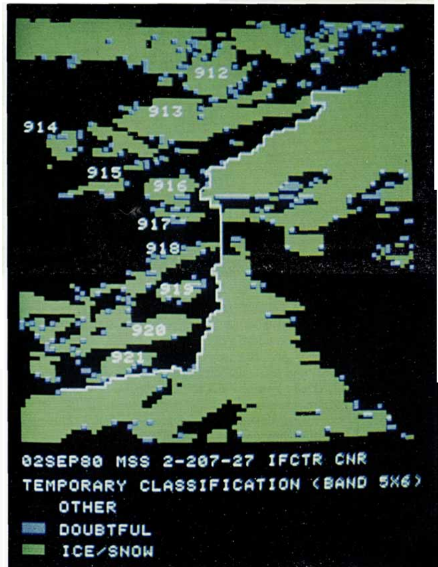
Figure 25. —Digitally processed Landsat 2 MSS image (2 September 1980; Path 207, Row 27) of part of the eastern Italian Alps. The Landsat image makes three classifications: other, doubtful, and ice/snow. This classifying represents the first step in the interpretation procedure developed to calculate glacier areas. The glaciers are labeled with their catalog reference numbers. The watershed line is superimposed from cartographic data. Image processing courtesy of the Istituto di Fisica Cosmica e Tecnologie Relative-CNR, Milan.
