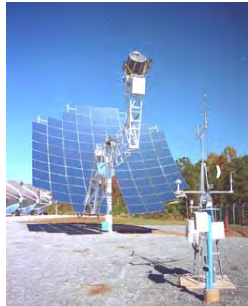
This parabolic dish collector in Shenandoah, Georgia, reflects sunlight to drive a Stirling heat engine, located on the arm above the dish. (Credit: Thomas Mancini, McDonnell Douglas/Sandia National Laboratories)
