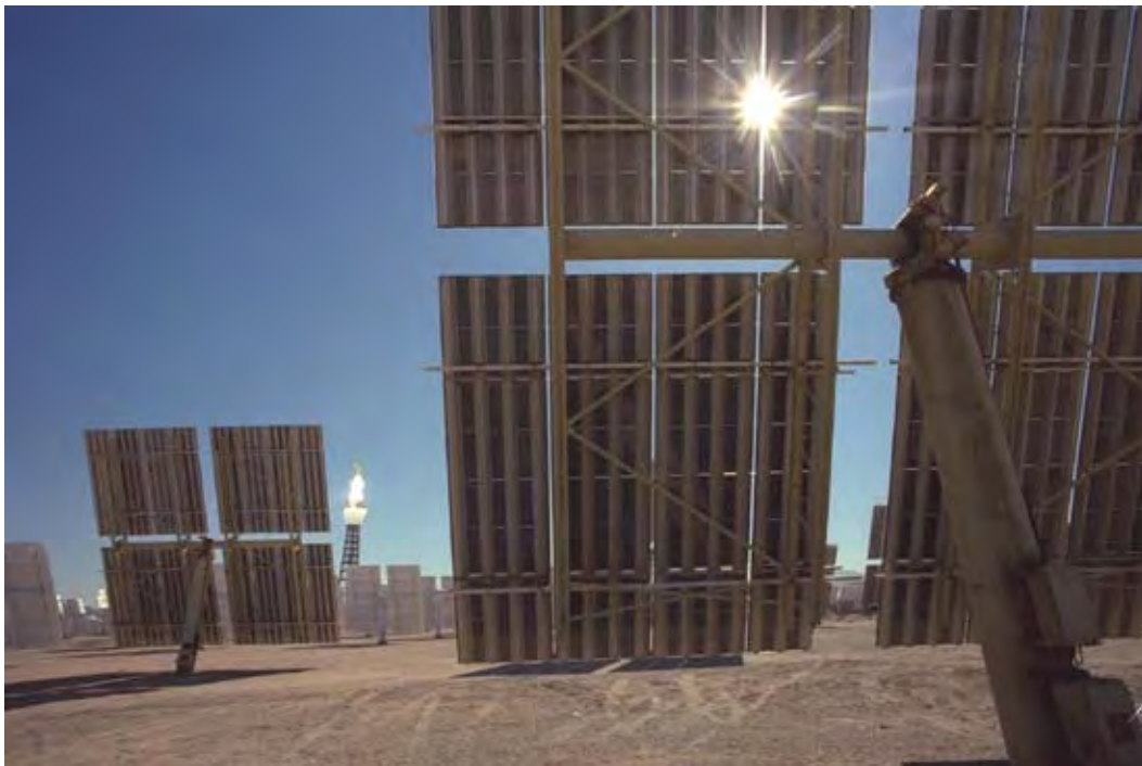
A central receiver tower generating electricity in the California desert, viewed from behind a heliostat. (Credit: James Pacheco, Southern California Edison/Sandia National Laboratories)
