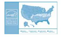
certain performance criteria. Since the energy efficiency performance of windows, doors, and skylights can vary by climate, product recommendations are given for four climate zones: a *mostly heating* zone (Northern), two *heating* and *cooling* zones (North/Central and South/Central); and a
