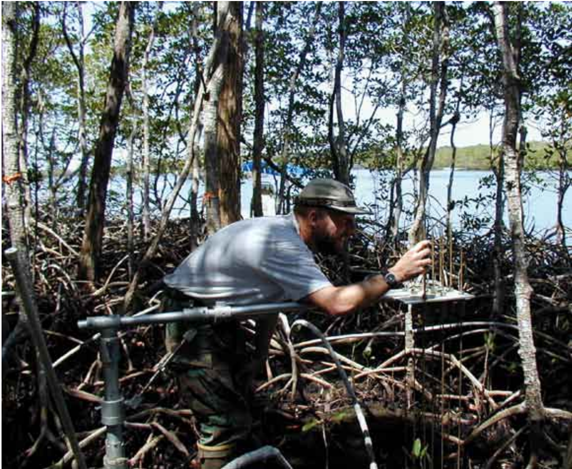
Man reading an original design Surface Elevation Table (SET) in the mangrove forests in Florida. Copyright: Donald Cahoon
